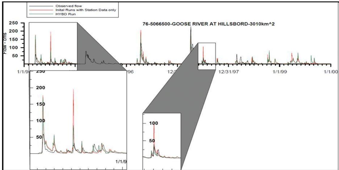
**Figure 7: Comparison of Hydrograph at the Goose River Using Station Data only and using HYBD Precipitation**
