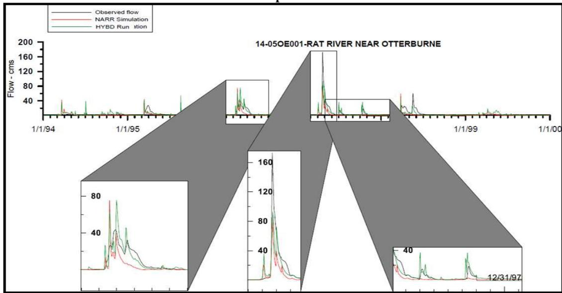
**Figure 8: Comparison of Hydrograph at the Rat River Using NARR Precipitation and using HYBD Precipitation**
